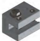
The S-5-H90 is a one-piece clamp that was developed to securely and cost-effectively accommodate metal roof panels with a horizontal seam greater than 0.65-in. Turning the clamp 90 degrees so that the bolt hole side is facing up, slip the clamp on the seam and tighten the setscrews.
