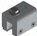
The S-5-V is a versatile clamp that fits vertical-folded seam profiles including most structural and architectural profiles. The clamps attach to the panel seam by tightening the round point stainless steel setscrews against the seam.
